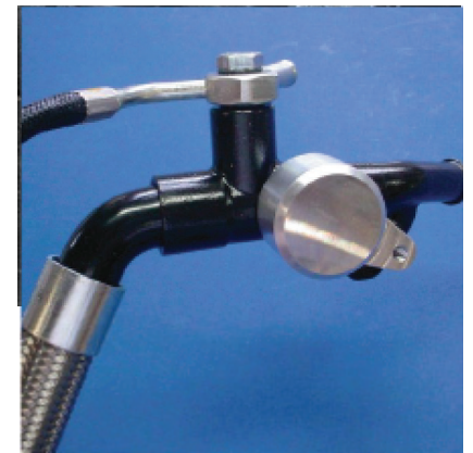
'13-'15 C&C Standpipe Cap Installed
